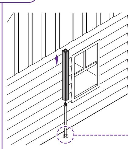
▶ Slide a post over the first pipe anchor. The post will rest on the edge of the anchor positioner.
