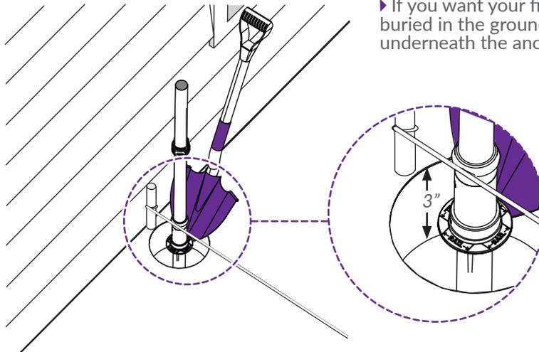
▶ If you want your finished fence post to appear buried in the ground, remove about 3" of soil from underneath the anchor positioner.
