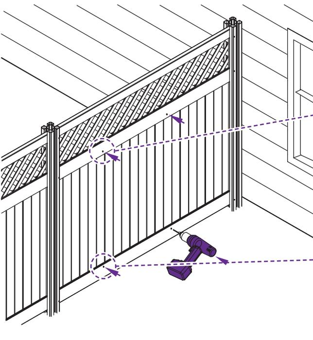
▶ Place (4) 1¼" Self-Drilling Stainless Steel Screws (I) in the middle and bottom rail
