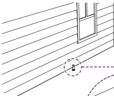
**Note:** Make sure your anchor positioner is level with the ground and not sloped at an angle.
