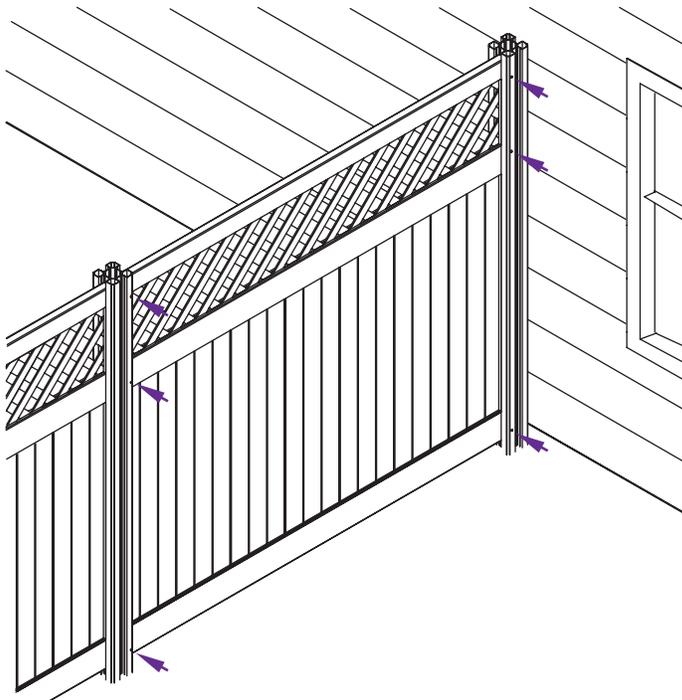
▶ Repeat this process for each end of the panel for a total of (6) screws per panel.
