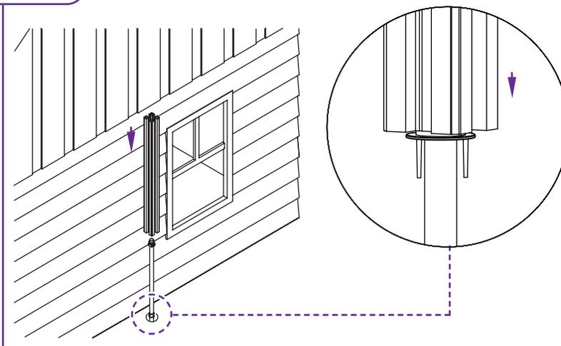
▶ Slide a post over the first pipe anchor. The post will rest on the edge of the anchor positioner.
