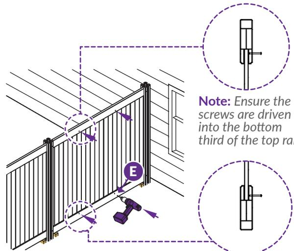
**Note:** Ensure the screws are driven into the bottom third of the top rail.
