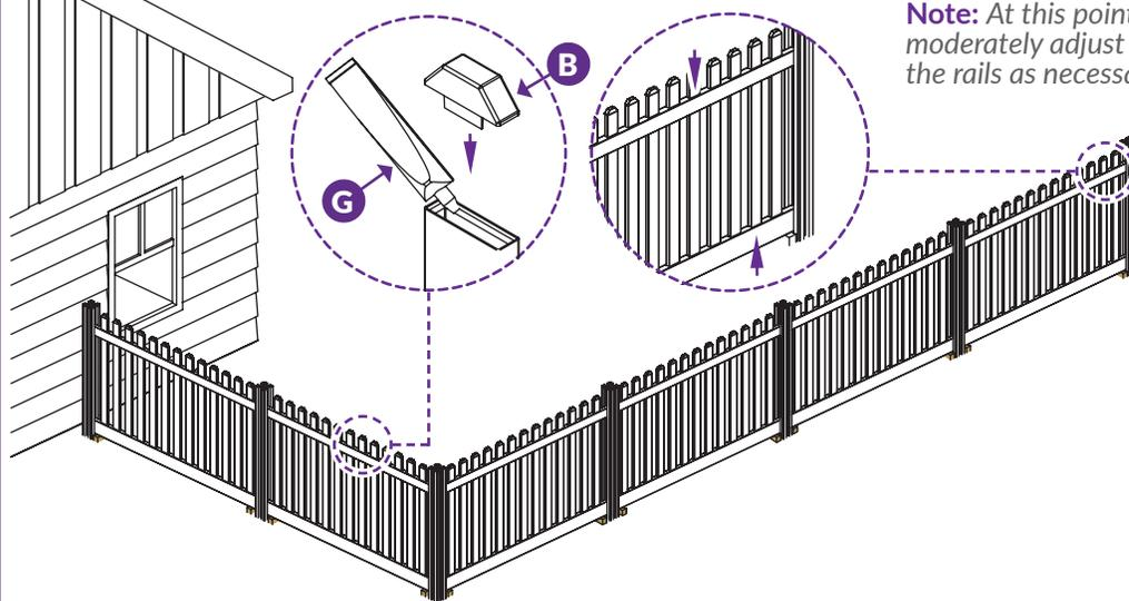
**Note:** At this point, you can moderately adjust the height of the rails as necessary.
