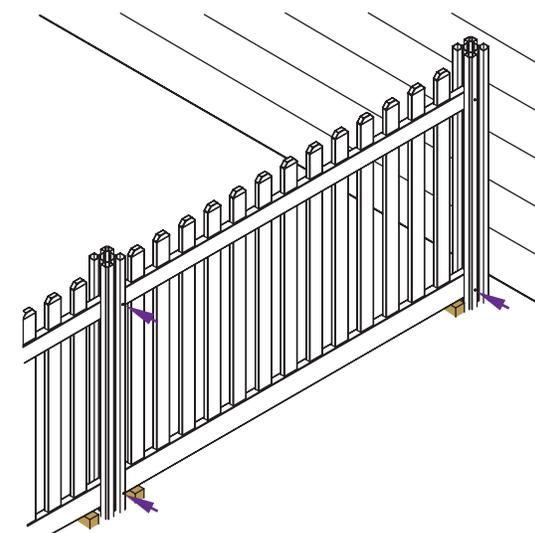
▶ Repeat in the remaining corners using (3) total 3½" self-drilling stainless steel screws.
