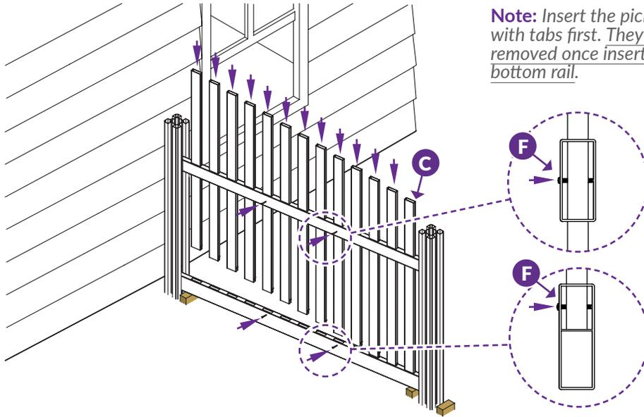
**Note:** Insert the picket ends with tabs first. They cannot be removed once inserted into the bottom rail.
