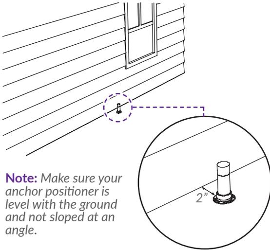
**Note:** Make sure your anchor positioner is level with the ground and not sloped at an angle.
