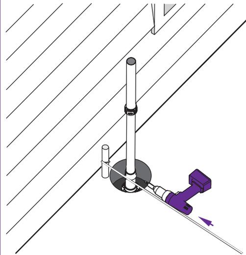
▶ Use (1) self-drilling tek screw to secure the anchor positioner to the pipe anchor.
