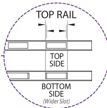
**Note:** Top rails have 2 different sized picket slots. Wider slots should be placed on the bottom side.
