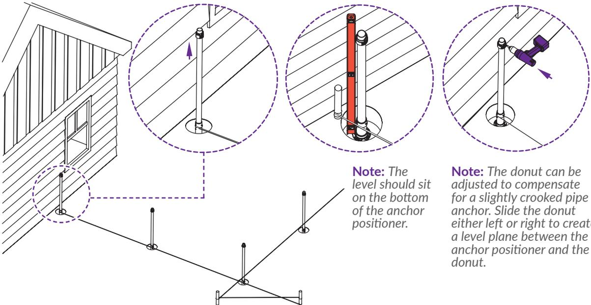
**Note:** The level should sit on the bottom of the anchor positioner.
