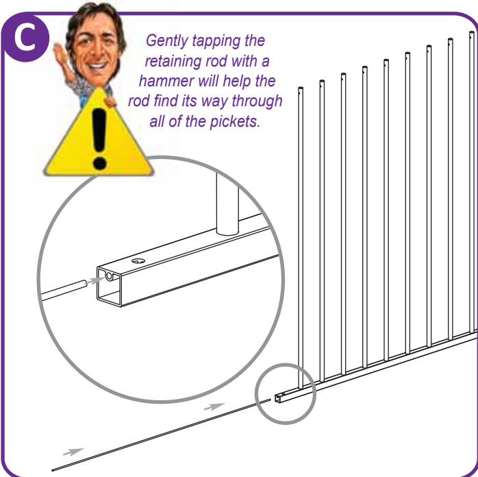
C - Insert retaining rod into one end of the bottom rail. Adjust vertical pickets one at a time to receive retaining rod. Turn in a clockwise, or counter clockwise motion as necessary while "threading" the retaining rod through the pickets.
